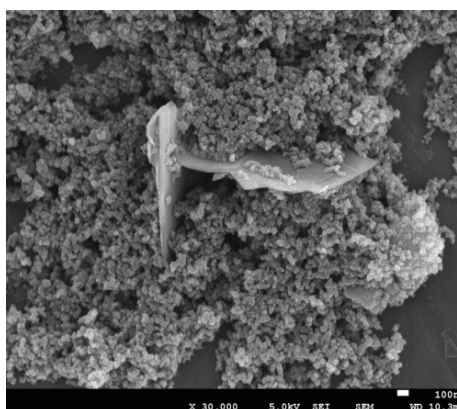
Figure 19 Electron microscope photo of graphene/carbon black composite
